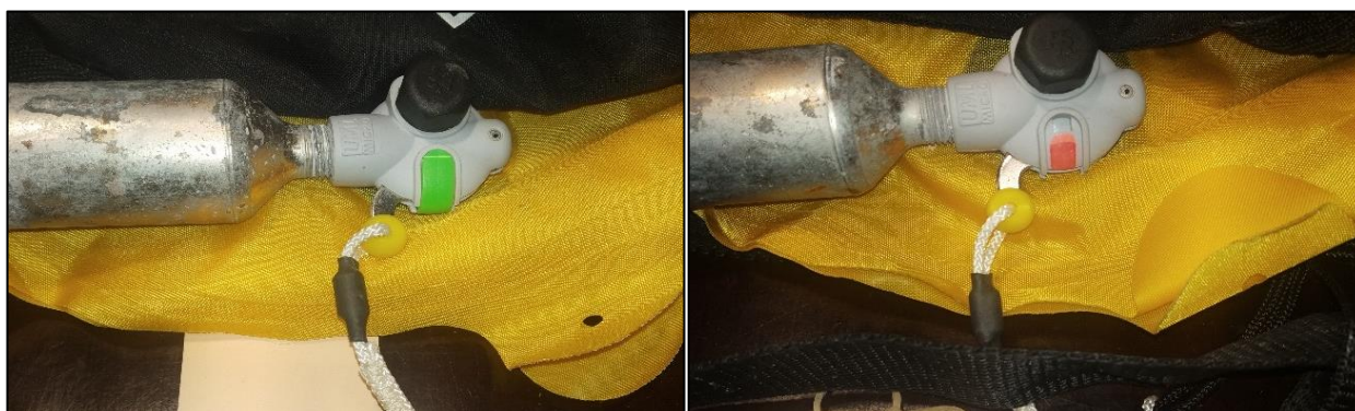
Figure 26: Inflation mechanism – Green Clip present (left); Green clip absent (right)
