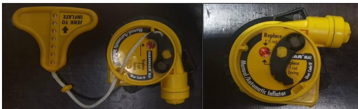
Figure 27: Hammar MA1 system with toggle intact (left) and toggle ripped off (right)
