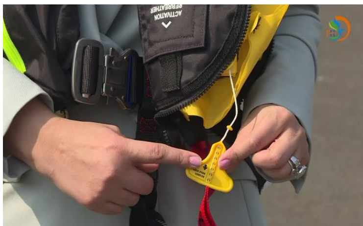
Figure 28: Hammer Toggle meant for ERBS
