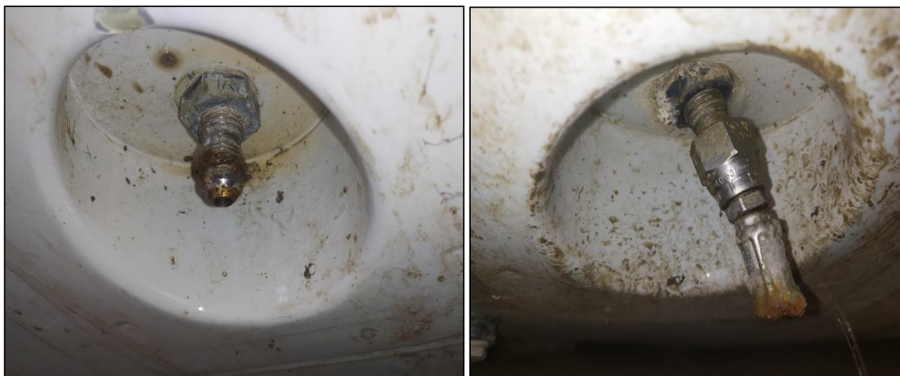
Figure 2: Aircraft side pneumatic connection to Life Raft Pods (left side and right side)
