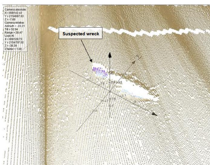
Figure 22: MBES 3D data image showing suspected wreck
